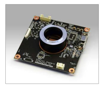
The core of the C13949-50U camera is the scientific image sensor, an advanced CMOS detector that simultaneously achieves high resolution, fast readout speeds and low noise. With its small size, board-level design and simple, low-cost integration using USB 3.0, the C13949-50U is the ideal camera for OEM scientific imaging.
